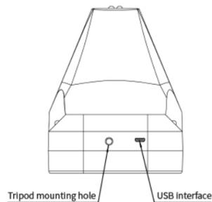
Tripod mounting hole USB interface
